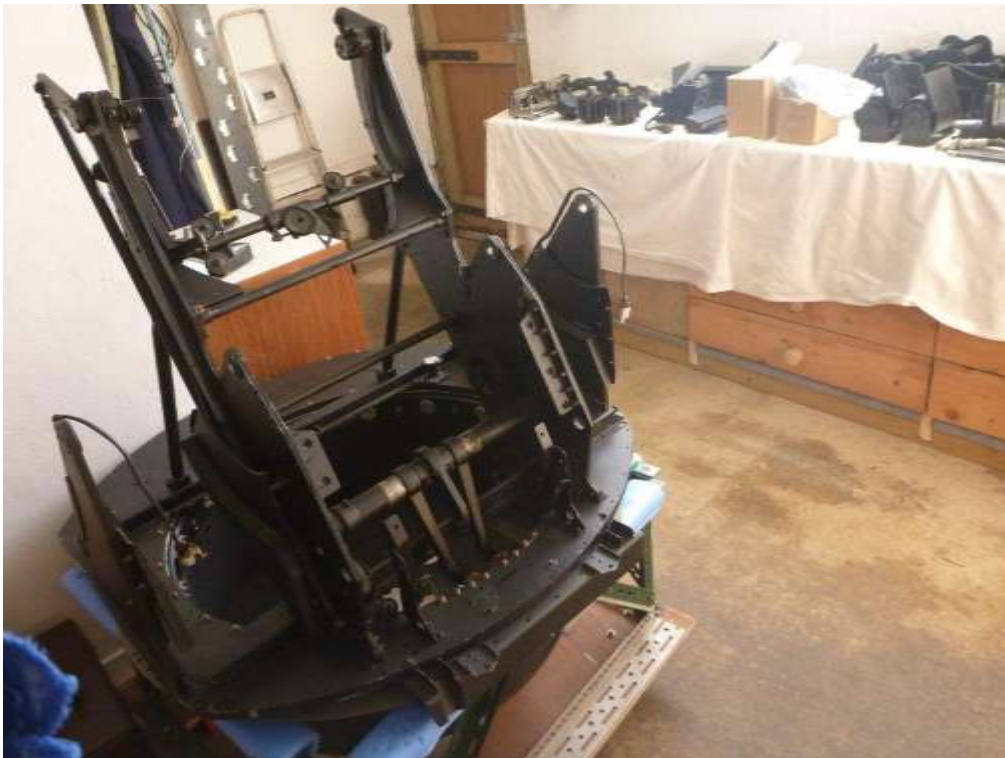
Turret rings, accommodation plate, superstructure and torque shaft.
