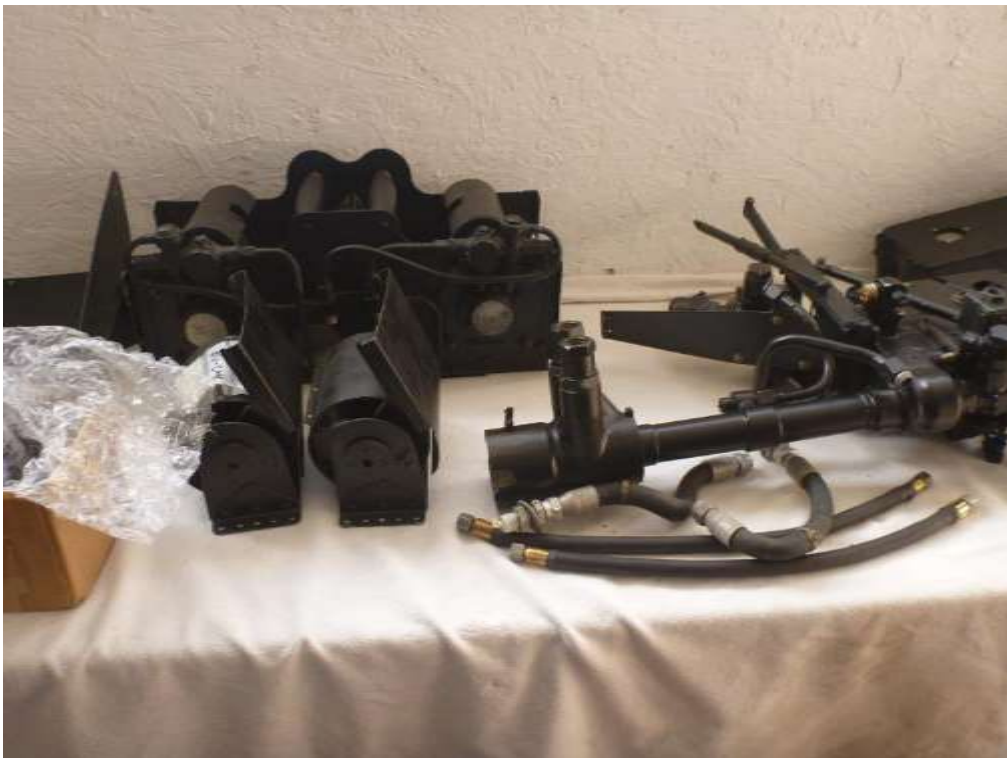
Ammunition servo feed and roller draught excluders.
