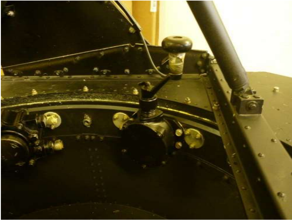
Seen below is the left-hand hydraulic rotation motor.
