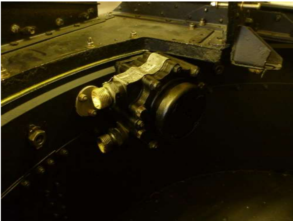
Seen below is the left-hand hydraulic rotation motor.
